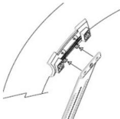
Step 2. Pull as much as possible on the steering wheel clamp as shown in the figure below, and then insert it into the holes so that it is fixed to a tight Use the two screws packed together to move tightly as shown in the figure below. Use a pair of scissors to cut the remaining clamping wheel clamp.
