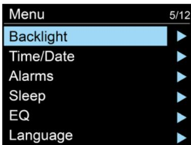
Select illuminated level of backlight (High/ Medium/ Low) and the duration of timeout (Always On/ 10/ 20/ 30/ 45/ 60/ 90/ 120/ 180 sec). With setting the timeout, the backlight will automatically change to dim if the device is not operated for the set amount of time.
