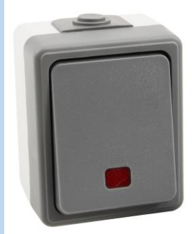
Orientierungs-Schalter McPower "Secure", 250V~/10A, IP44, AP, grau 1534947
